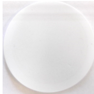
Figure 7: Filter pad LP feedwater 2.5 months after beginning Anodamine HPGF treatment
