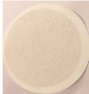
Figure 6: Filter pad LP feedwater pre-Anodamine HPGF treatment
