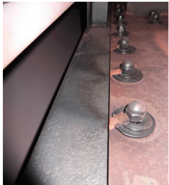
Figure 3: Localized two-phase FAC
